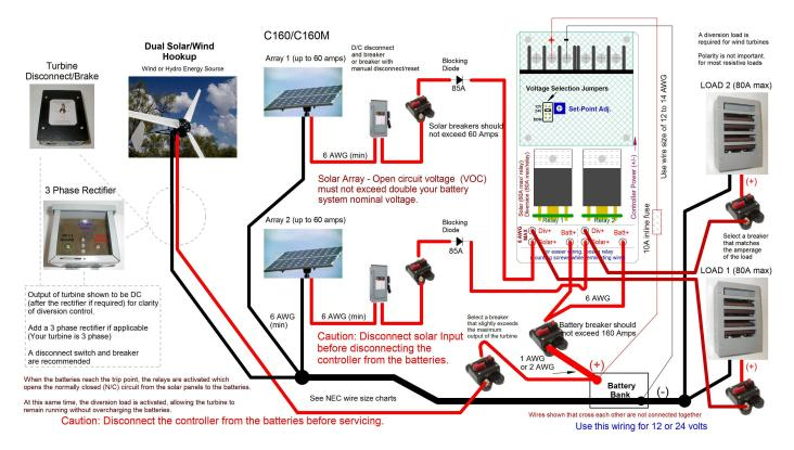
Simply combine the hookup instructions of the two earlier diagrams to complete the terminations for the dual solar/wind hookup.
