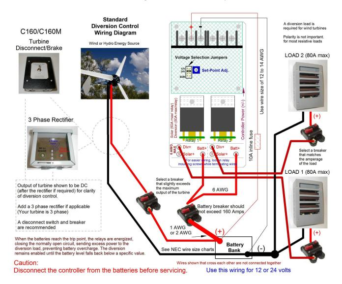
This wiring is for turbines, and is the most common setup for the C160/C160M controller. To use this wiring:
