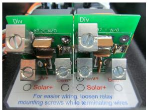
Relay Termination Blocks (2 relays, with 3 terminals each)
