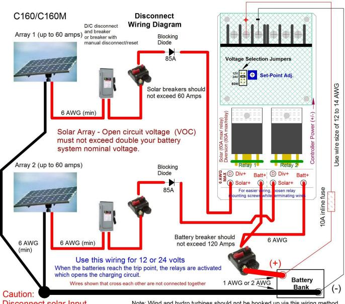
Disconnect solar Input before disconnecting the controller from the batteries.
