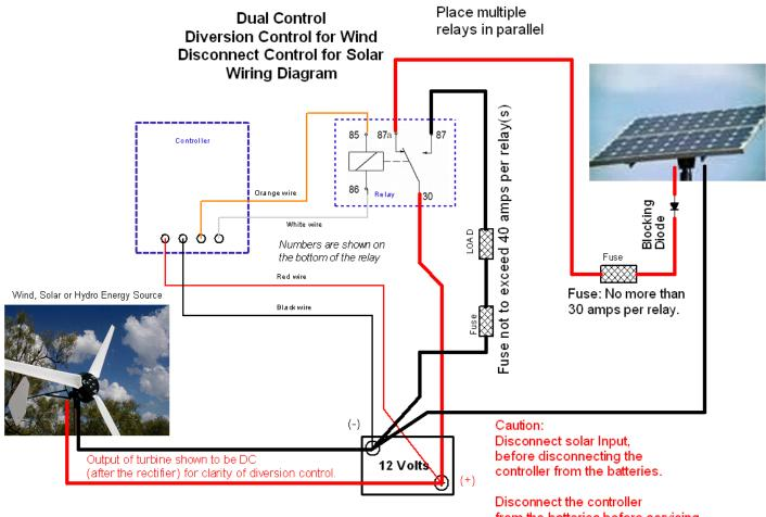
When the batteries reach the trip point, the relay is activated which opens the N/C circuit from the solar panels into the batteries.
