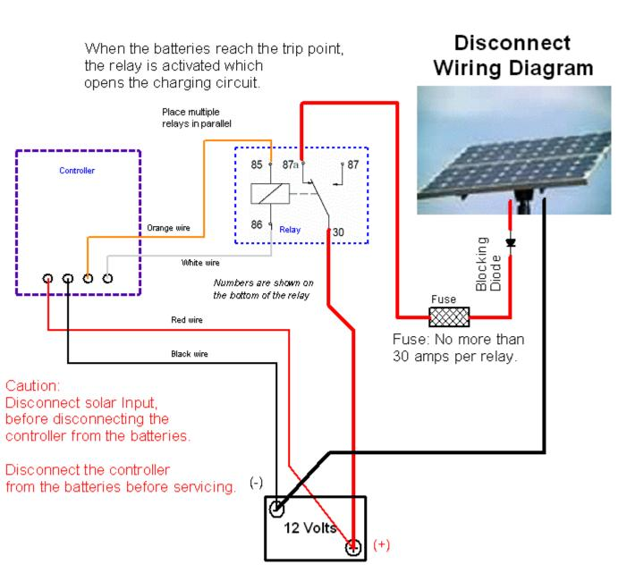
Note: Wind and hydro turbines should not be hooked up via this wiring method as they normally need to remain under a load while operating.
