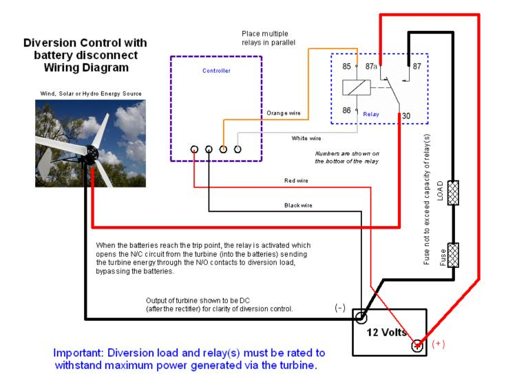
This wiring method is similar to the standard diversion control wiring, except that when the trip point is reached, power from the charge source (wind/solar etc) is no longer allowed to reach the batteries, but instead is sent directly to the diversion load. Use this method if you want your turbine to see a larger load when the batteries are full, possibly causing a slow down in your turbine RPM. Please see the notes about diversion philosophy in the earlier portions of this manual.
