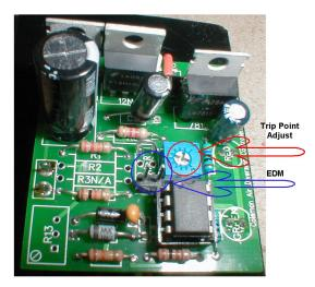
**EDM:** The two-pin jumper allows for enabling EDM. As shipped, this jumper will be hanging on one terminal only. We have shipped it in this manner so the jumper is available to you but not actually being used. To enable EDM, place the small black jumper across both of the pins extending from the PCB.
