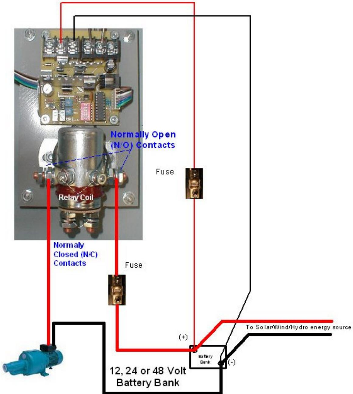
In this mode, the D/C input to the pump will only be connected if and when the battery reaches the user settable upper trip point.
