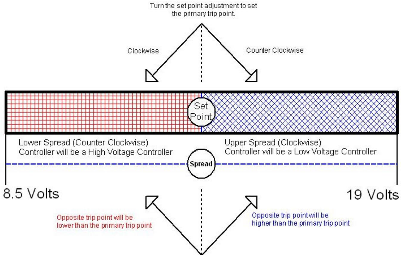
Voltages reflect a 12-volt system; double this for 24-volt systems, quadruple for 48-volt systems.
