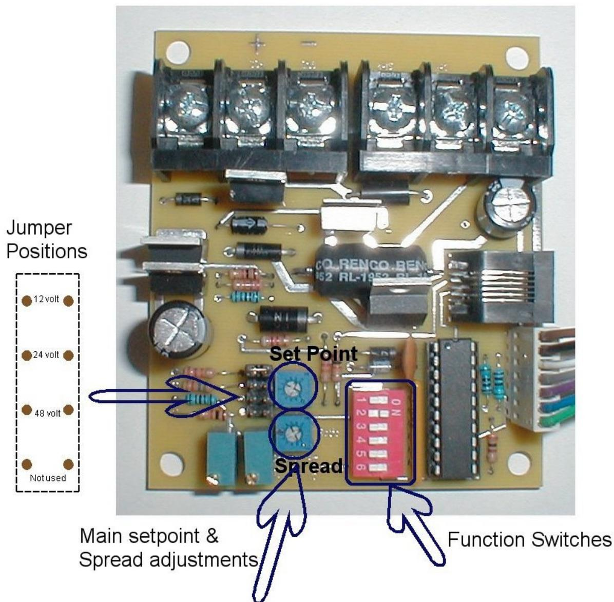
The voltage jumper block allows you to configure the controller for a 12, 24 or 48 volt battery bank. Please move the jumper as necessary, to match your battery bank.
